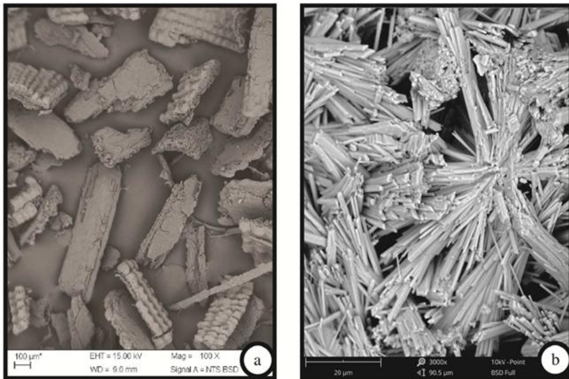
Fig. 1 - (a) rice husks after grinding process by UNIFEI MEV (b) gypsum crystals after their hydration by scanning electron microscopy by the bench MEV.
