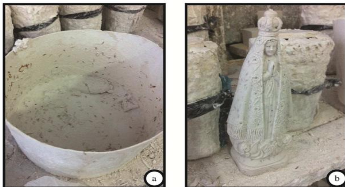
Fig. 3 - Mixture of composite (a) and artifacts developed with gypsum and in-nature rice husks (b) at JB company.
